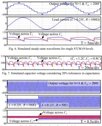
Fig. 8. Simulated waveforms for step load change.
